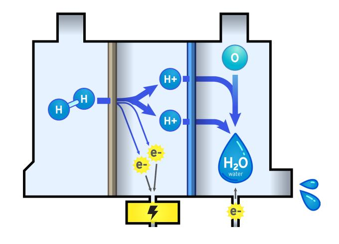
The fuel cell separates electrons from hydrogen molecules. The electrons generate electricity to charge the battery while the remaining hydrogen ions combine with oxygen to create water.
