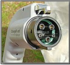
SAE J1772 Standard Level 1 & 2 Charging Connection (Left) and Plug (Right) US EVs
