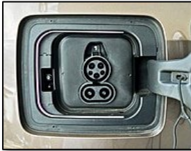
SAE Combined Charging System (CCS1) (Left) Standard Level 1 and 2 AC EV and DC Fast Charging connection and Plug (Right) - US EVs
