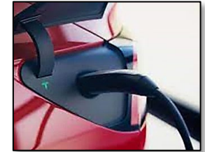
Tesla EV Connector (Left) and Plug (Right), Recently approved as SAE J3400 or North American Charging Standard (NACS)
