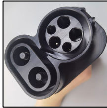
SAE Combined Charging System (CCS1) (Left) Standard Level 1 and 2 AC EV and DC Fast Charging connection and Plug (Right) - US EVs
